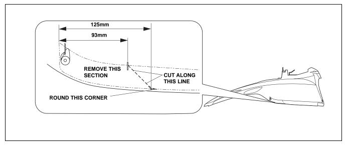
2. **Belly Pan Modification:** Remove a section of both right-hand (RH) and left-hand (LH) sides of the belly pan as shown in the illustration below. Take care not to remove excess material to avoid a gap between the hood and belly pan.
